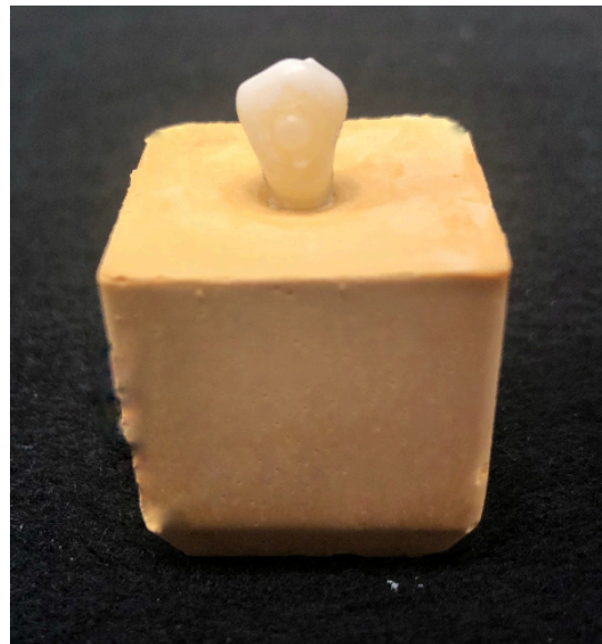
Figure 23. Sample tooth mounted in microstone block
