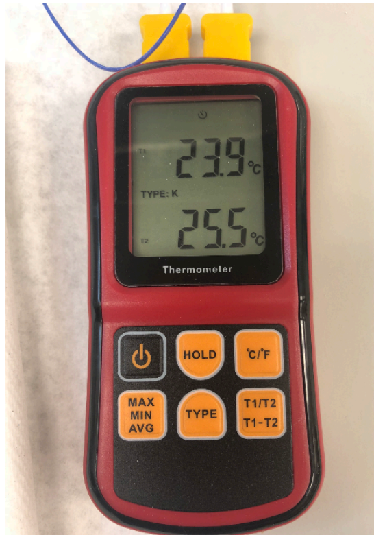
Figure 24. Liumy Tools K-type thermocouple
